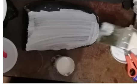
Figure 6. Application of the mold release wax.
