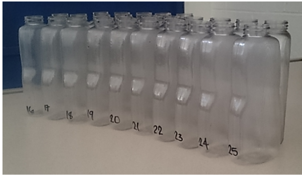
Figure 8. Plastic bottles made with the use of printed molds.
