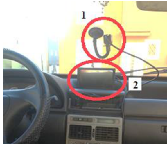
Figure 4. System of traffic sign detection in Ecuador, for the Stop, Give-way and Speed (50 and 100) signs, installed on the windshield of an experimental vehicle.
