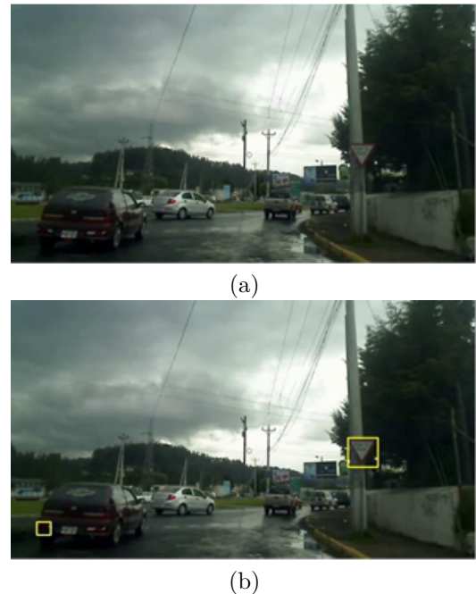
Figure 7. Results of the traffic sign detection system in the case of Stop signs, during a sunny day on a highway; (a) input image, (b) ROI and (c) detections.
