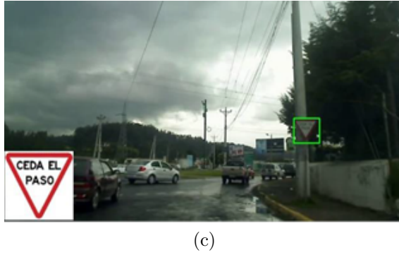
Figure 8. Results of the traffic sign detection system in the cases Stop and Give-way signs, during a dark day in an urban area; (a) input image, (b) ROI and (c) detections.
