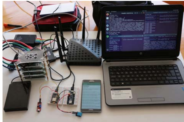
Figure 4. Setup for tests: from left to right it is observed a cluster of 3 Raspberry Pi running all services on Docker; an ESP8266 monitoring the level of noise with an KY038; an MKR1010 monitoring ambient temperature with an DHT11; an N9005 injecting random messages, and a laptop monitoring all services.
