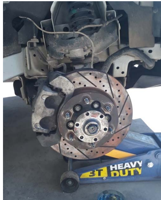
Figure 10. Implementation of the ventilated disc
