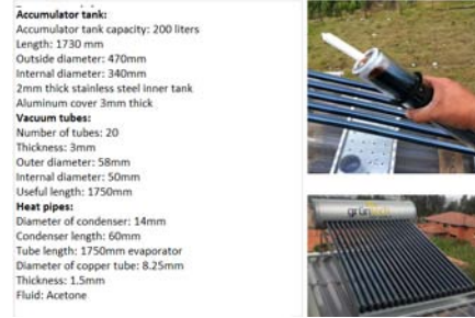
Figure 15. Characteristics of solar heaters installed
