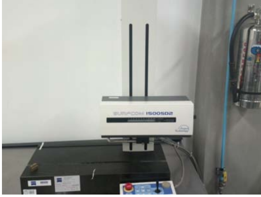
Figure 4. CARL ZEISS rugosimeter model SURFCOM 1500SD2.
