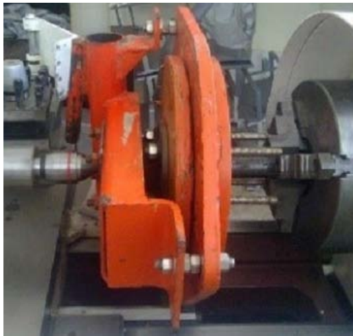
Figure 11. Assembly of the generator on the lathe.
