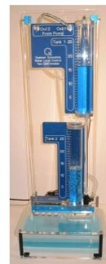
Figure 3. Coupled tank system
