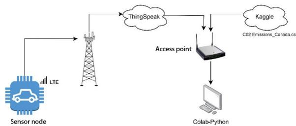
**Figure 1.** IoT Architecture for Pollutant Gas Monitoring.
