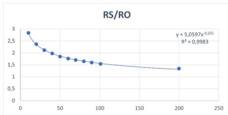
Figure 3. Calibration Curve of the MQ-135 Sensor.
