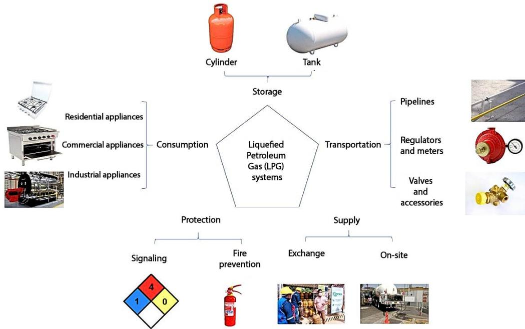
Figure 1. General diagram of an LPG system. Adapted from [31]
