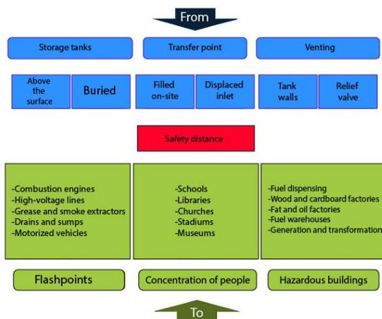
**Figure 3.** Criteria for locating stationary containers based on safety distance [27]
