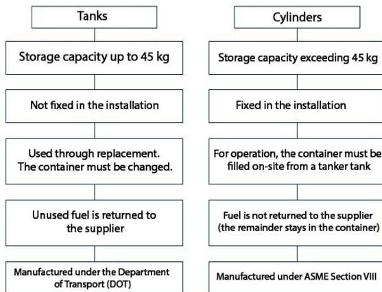
Figure 2. Differences between cylinders and tanks. Adapted from [32, 33]
