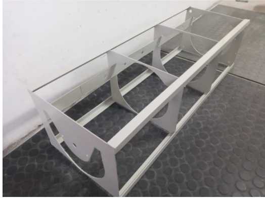
Figure 9. Metallic structure that supports the microgeneration system
