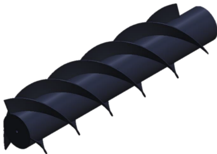
Figure 3. Archimedes screw hydraulic microturbine
