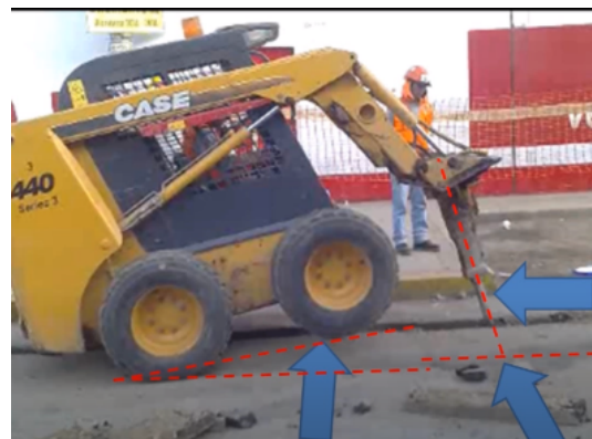
Figure 3. Skid Steer working with Hydraulic Hammer SB202 [16]
