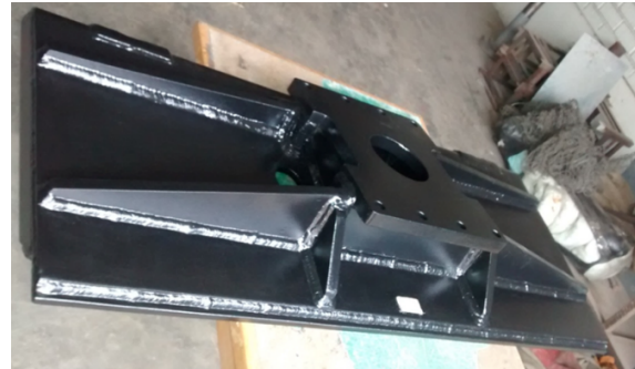
Figure 15. Adapter plate as final product
