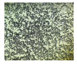
Figure 13. Lactose particles grinded for 1 h – Scale 100  $\mu m$
