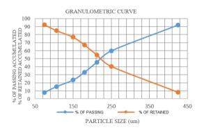
Figure 7. Percentage of passing accumulated and retained accumulated *vs.* particle size
