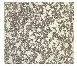
Figure 12. Lactose particles grinded for 5 h – Scale 50  $\mu m$
