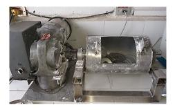
Figure 4. Horizontal rotating mill
