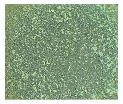
Figure 14. Lactose particles grinded for 5 h – scale 100  $\mu m$
