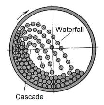
Figure 1. Movement of the load in a ball mill [5]
