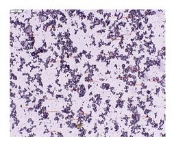
Figure 11. Lactose particles grinded for 1 h – Scale 100  $\mu m$
