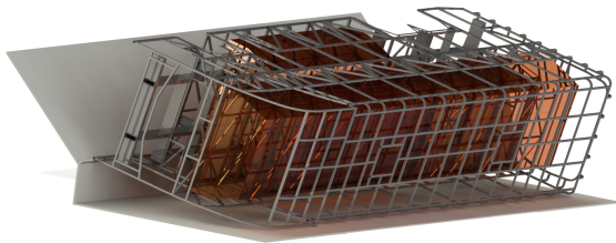
Figure 5. Bus in position of first contact with the rigid impact surface
