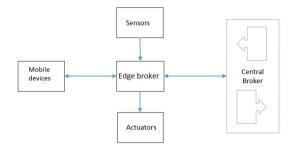
**Figure 1.** Components in the local or edge layer of the IoT system
