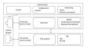
Figure 2. Components in the centralized layer of the IoT system
