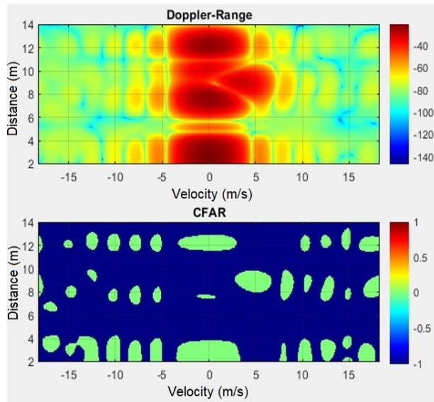
Figure 12. Range-Doppler map in dB and result of CFAR
