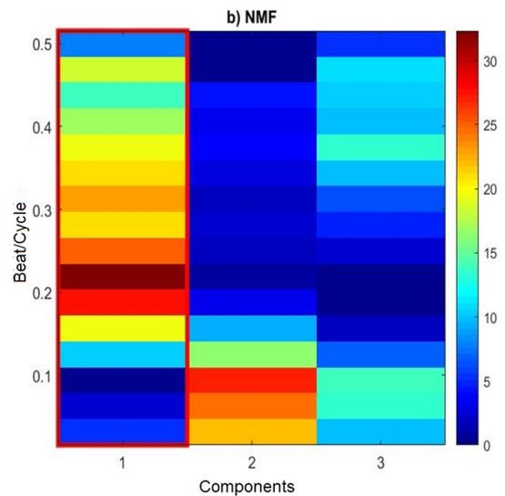
**Figure 8.** Component with the greatest TWA magnitude of the TWADB12 signal, the TWA is calculated at 0,5 bcpl.
