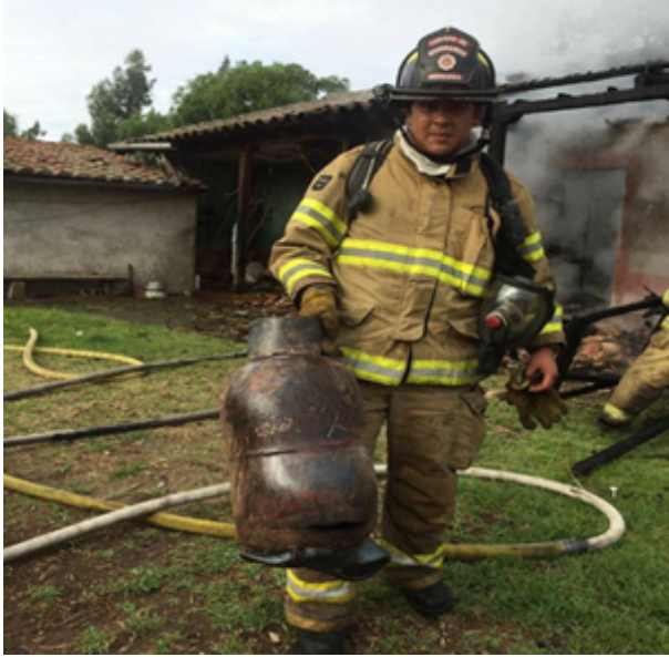
Figura 4. LPG cylinder that has suffered BLEVE [27].
