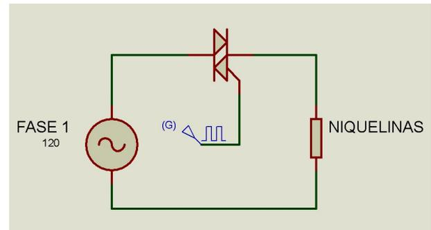
Figure 1. Simulation scheme of the AC/AC converter.
