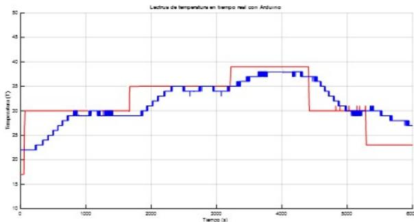
Figure 10. Operation of the ON/OFF control with PID.
