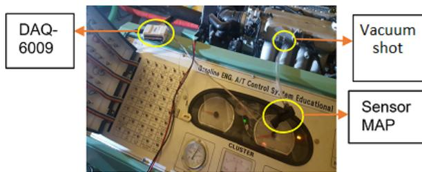
Figure 2. Connection of the MAP sensor.
