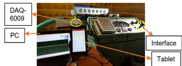
Figure 1. Engine instrumentation.
