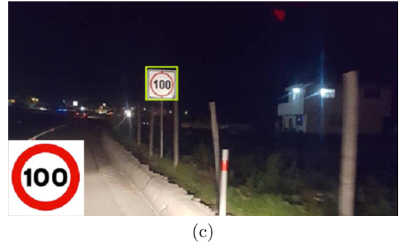
Figure 10. Results of the traffic sign detection system in the case of Speed of 100, during a dark day in urban area; (a) input image, (b) ROI and (c) detections.
