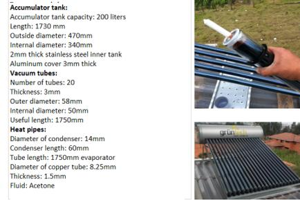
Figure 15. Characteristics of solar heaters installed
