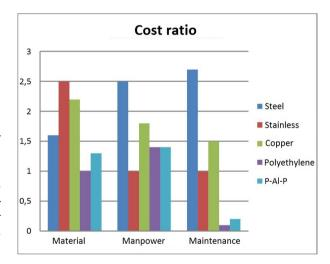
Figure 4. Ratio of pipe costs for LPG services.
