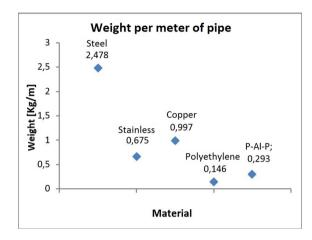
Figure 3. Comparison of pipe weights for conducting LPG
