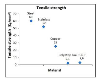
Figure 1. Comparison of tensile strength
