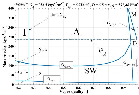
**Figure 3.** Flow pattern map for test A for the R600a refrigerant with  $T_{\text{sat}} = 6,756 \text{ }^{\circ}\text{C}$ ,  $D = 3,8 \text{ mm}$ ,  $q = 391,44 \text{ W}\cdot\text{m}^{-2}$  and  $G_A = 236,5 \text{ kg}\cdot\text{m}^{-2}\cdot\text{s}^{-1}$
