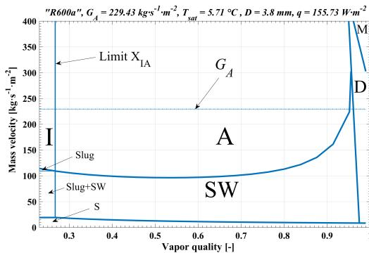
**Figure 6.** Flow pattern map for test B for the R600a refrigerant with  $T_{sat} = 5.71 \text{ }^{\circ}\text{C}$ ,  $D = 3.8 \text{ mm}$ ,  $q = 155.73 \text{ W}\cdot\text{m}^{-2}$  and  $G_A = 229.43 \text{ kg}\cdot\text{m}^{-2}\cdot\text{s}^{-1}$
