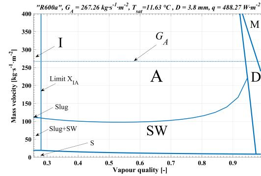
**Figure 4.** Flow pattern map for test B for the R600a refrigerant with  $T_{\text{sat}} = 11,63 \text{ }^{\circ}\text{C}$ ,  $D = 3,8 \text{ mm}$ ,  $q = 488,27 \text{ W}\cdot\text{m}^{-2}$  and  $G_A = 267,26 \text{ kg}\cdot\text{m}^{-2}\cdot\text{s}^{-1}$
