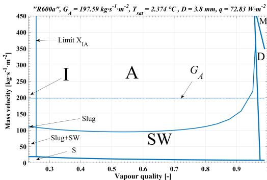
**Figure 7.** Flow pattern map for test E for the R600a refrigerant with  $T_{sat} = 2.374 \text{ }^{\circ}\text{C}$ ,  $D = 3.8 \text{ mm}$ ,  $q = 72.83 \text{ W}\cdot\text{m}^{-2}$  and  $G_A = 197.59 \text{ kg}\cdot\text{m}^{-2}\cdot\text{s}^{-1}$
