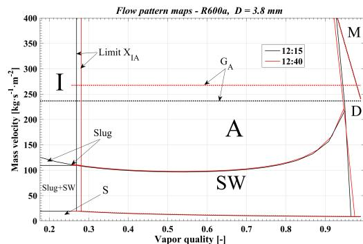
**Figure 8.** Comparison of the maps corresponding to tests A and B at 12:15 and 12:40, respectively
