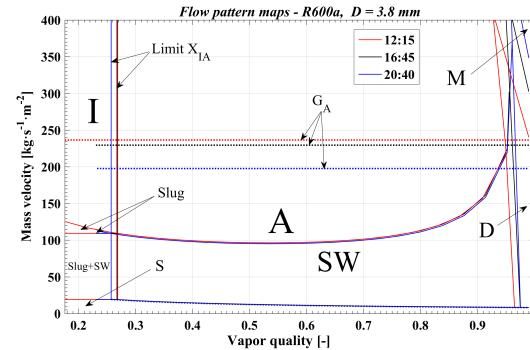
**Figure 12.** Comparison of the flow pattern maps with incident solar radiation at different times
