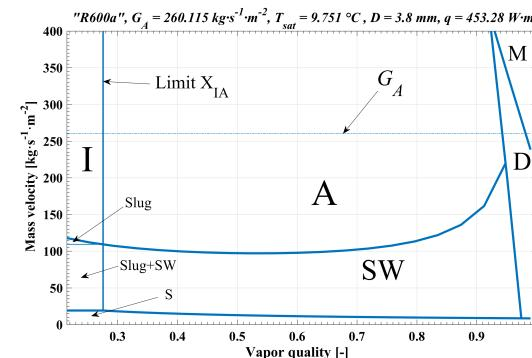
**Figure 5.** Flow pattern map for test C for the R600a refrigerant with  $T_{\text{sat}} = 9,751 \text{ }^{\circ}\text{C}$ ,  $D = 3,8 \text{ mm}$ ,  $q = 453,28 \text{ W}\cdot\text{m}^{-2}$  and  $G_A = 260,115 \text{ kg}\cdot\text{m}^{-2}\cdot\text{s}^{-1}$
