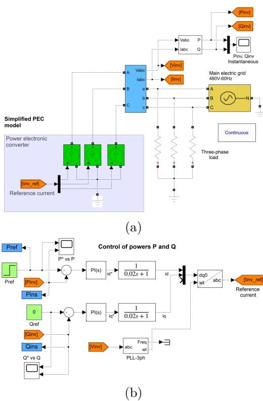
**Figure 11.** Implementation scheme of the simplified model:
