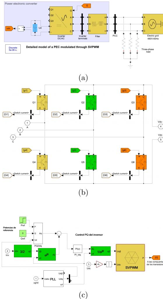
**Figure 5.** Implementation of the PEC in MATLAB/Simulink® (detailed model): a) test electric system; b) inverter configuration and; c) PQ controller and SVPWM modulator
