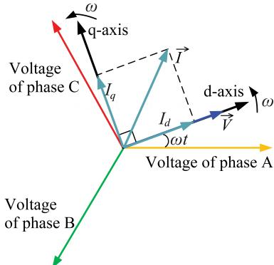
**Figure 4.**  $d - q$  coordinate system
