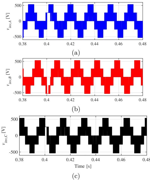
**Figure 6.** Three-phase generated at the inverter terminals
