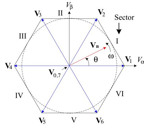
**Figure 3.** SVPWM modulation
