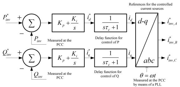
**Figure 10.** Proposed simplification for the PQ controller
