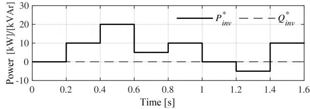
**Figure 13.** Power set-point signals applied to the converter
