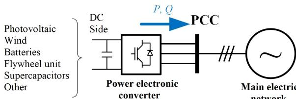
**Figure 1.** Power electronic converter connected to the grid
