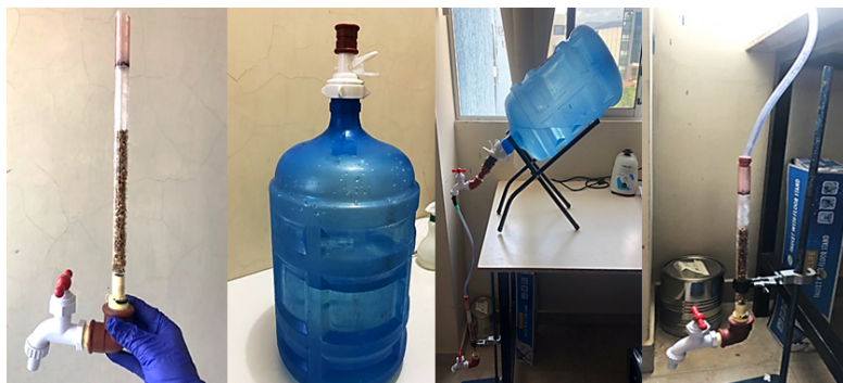
Figure 1. Diatoms were placed on a glass support which was connected to a faucet at one end and to a drum at the other.
