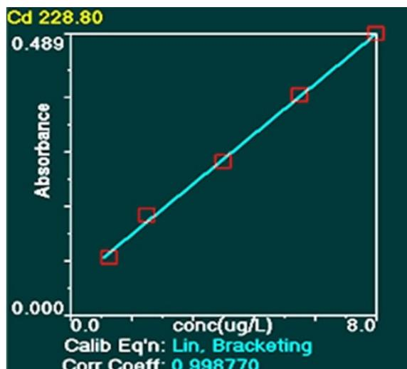
Figure 3. Linear range obtained by the equipment
