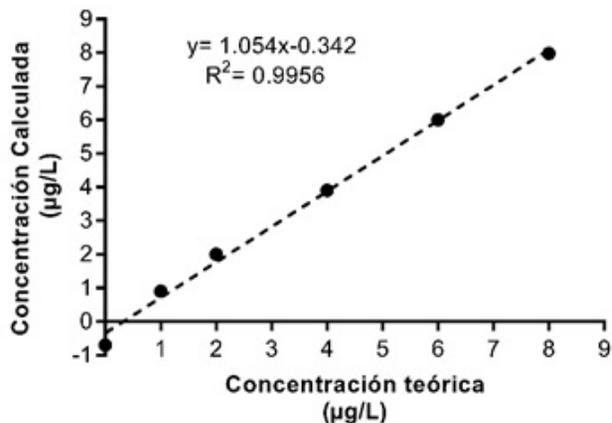
Figure 2. Linear range of the method 0-8 ppb.
