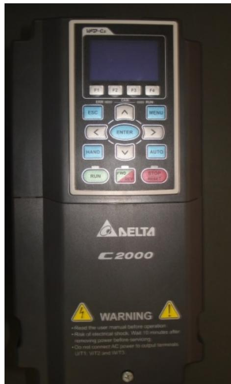
Figura 5. 3-phase frequency inverter.
