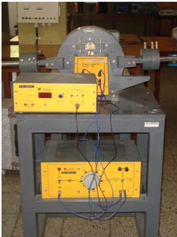
Figure 12. Electromagnetic brake.
